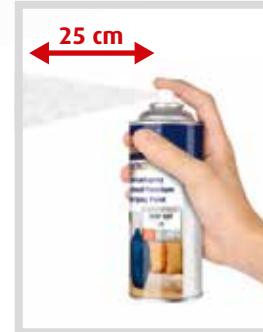
Always hold the spray paint can vertically when spray painting. Test spray first to check the colour shade. The correct spray distance is 25 cm. Always start spraying away from the object.
