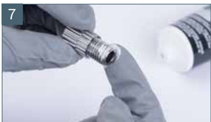
Grease thread of material flow control screw
