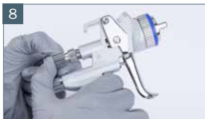
Install material flow control screw
