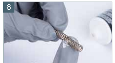
Grease and insert paint needle spring
