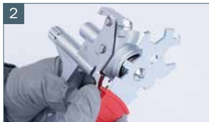
Tighten fluid tip by hand using the universal spanner.
