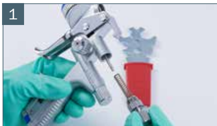
1 First remove paint needle.
